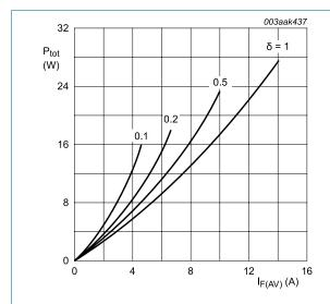
$$\begin{split} & I_{\text{F(AV)}} = I_{\text{F(RMS)}} \times \sqrt{\delta} \\ & V_{\text{o}} = 1.300 \text{ V}; \text{ R}_{\text{s}} = 0.050 \text{ }\Omega \end{split}$$
