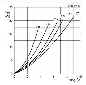
a = form factor =  $I_{F(RMS)}/I_{F(AV)}$  $V_o$  = 1.300 V;  $R_s$  = 0.050  $\Omega$
