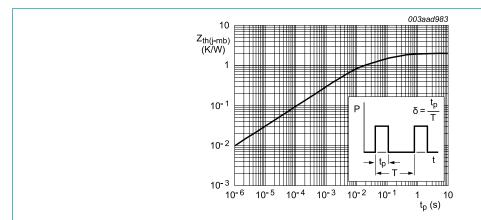
Fig. 3. Transient thermal impedance from junction to mounting base as a function of pulse width
